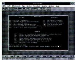
QmodemPro's main screen offers a toolbar, status bar and macro buttons. You can copy text from the main display window during a session.
